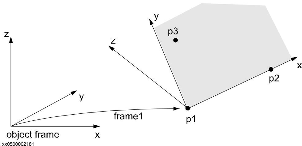
Three positions, p1- p3 related to the object coordinate system are used to define the new coordinate system, frame1. The first position, p1, is defining the origin of the new coordinate system. The second position, p2, is defining the direction of the x-axis. The third position, p3, is defining the location of the xy-plane. The defined frame1 may be used as a displacement frame, as shown in the example below:
