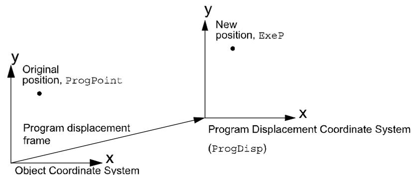
Program displacement is activated when the instruction PDispOn is executed and remains active until some other program displacement is activated (the instruction PDispSet or PDispOn) or until program displacement is deactivated (the instruction PDispOff).
