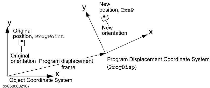
The program displacement is automatically reset
