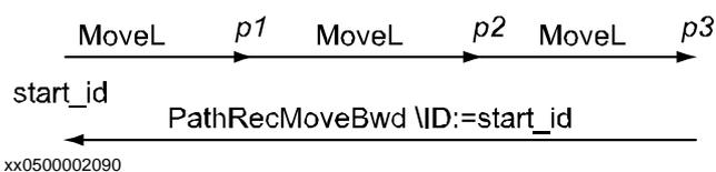
The example above will start the path recorder and the starting point will be tagged with the path identifier start\_id. Thereafter, the robot will move forward with traditional move instructions and then move back to the start position again using the recorded path. To be able to run PathRecorder move instructions, the path level has to be changed with StorePath.
