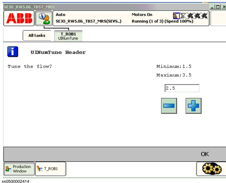
Above numeric tune message box with icon, header, message, init-, increment, max-, and minvalue are written on the FlexPendant display. The message box checks that the operator tune the flow value with step 0.1 from init value 2.5 is within the value range 1.5 .. 3.5. Program execution waits until OK is pressed and then the selected numerical value is returned and stored in the variable flow.
