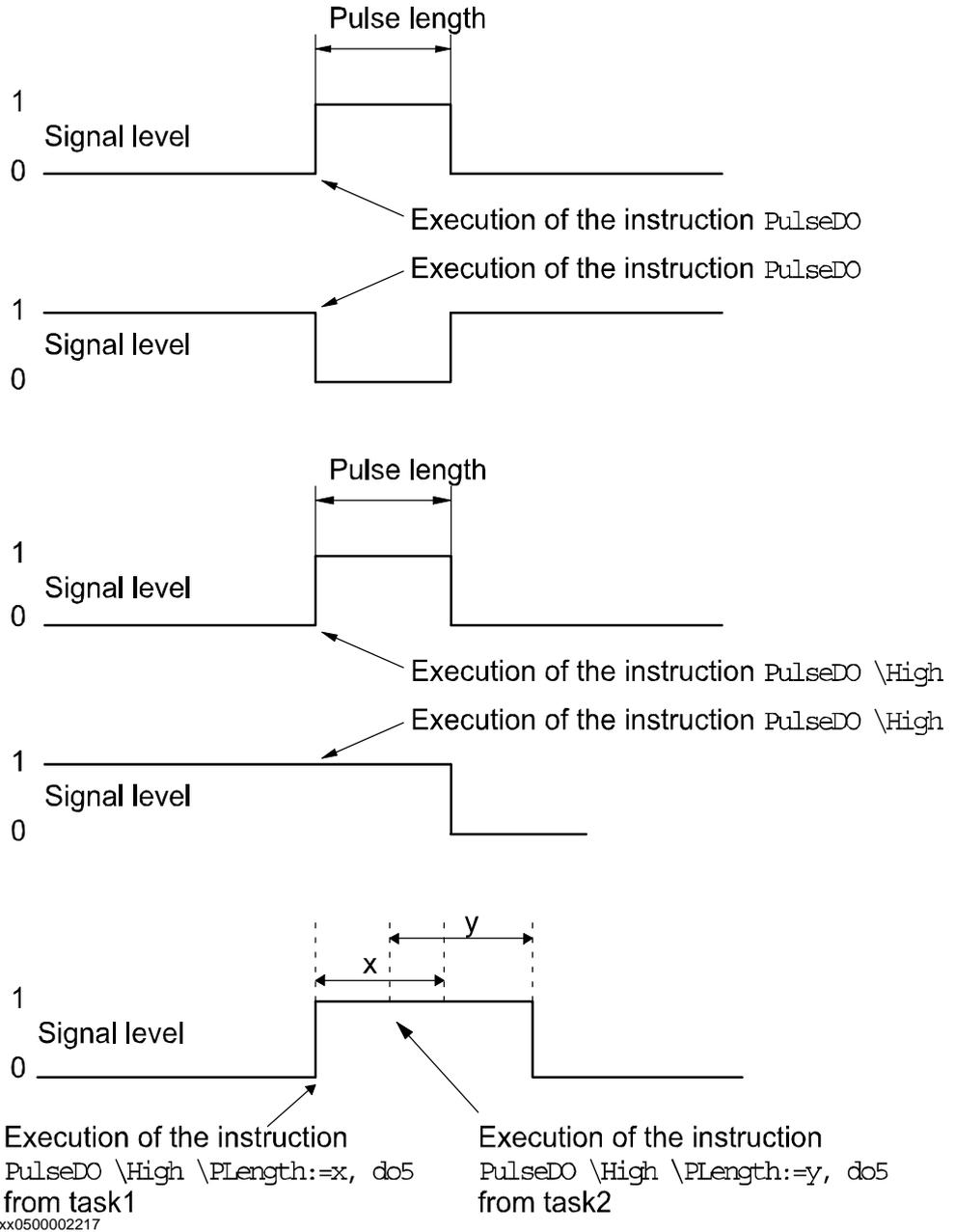
The next instruction is executed directly after the pulse starts. The pulse can then be set/reset without affecting the rest of the program execution.
