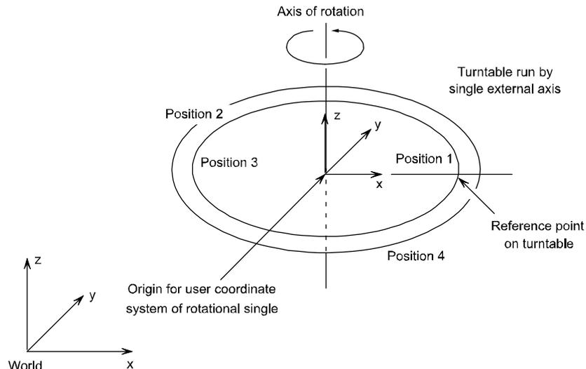
The user coordinate system for the rotational axis has its origin in the center of the turntable. The z direction coincides with the axis of rotation and the x axis goes through the reference point.
