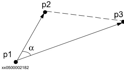
The triangle is not considered to be well shaped if the angle  $\alpha$  is too small. The angle  $\alpha$  is too small if:
