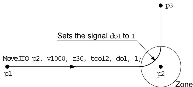
For stop points we recommend the use of “normal” programming sequence with `MoveJ` + `SetDO`. But when using stop point in instruction `MoveJDO`, the digital output signal is set/reset when the robot reaches the stop point.
