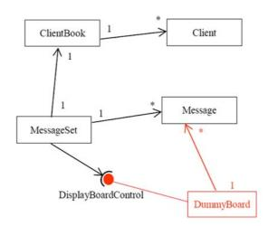
Note the use of the concise "ball and socket" notation for the DisplayBoardControl interface.
