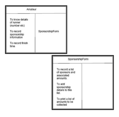
Having developed CRC cards we can role-play a range of scenarios in order to check the system works 'on paper'. If not we can amend the design before getting into the time consuming process of programming a flawed plan.
