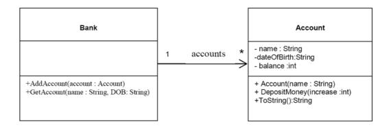
The diagram above represents the basics of a banking system (admittedly a very simplistic banking system). In this system a class is used to simulate a Bank and maintain a collection of Accounts... for the moment we will use a List to manage this collection.
