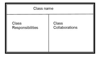
Responsibilities are the things the class needs to know about (ie the attributes) and the things it should do (ie. the methods) though on a CRC card these are not as precisely defined as on a UML diagram. The collaborations are other classes that this class must work with in order to fulfil its responsibilities.
