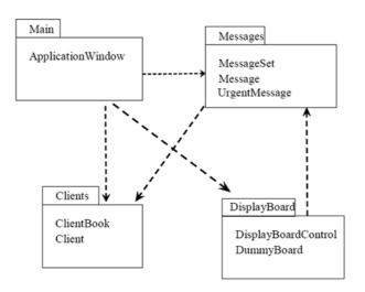
This diagram shows the four packages used and the classes within each package. Also shown are associations between the packages. Not surprisingly the main package, which houses the system interface, is associated with all of the other packages – this is because the interface invokes functionality throughout the system.
