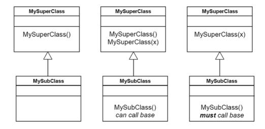
On the left above:- it is legal, though bad practice, to have a subclass with no constructor because superclass has a parameterless constructor.
