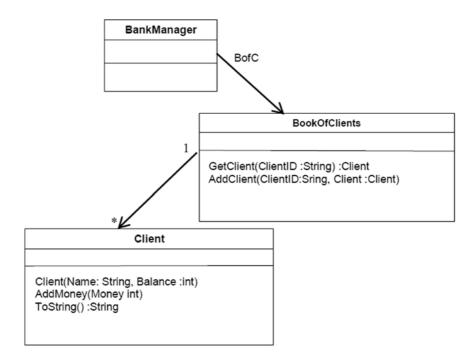
In this system a BankManager class maintains a book of clients (BofC). Client objects can be added by the AddClient() method which requires an ID for that client and the client object to be added. Clients can be retrieved via the GetClient() method which requires a ClientID as a parameter and returns a client object (if one exists) or generates an exception (if a client with the specified ID does not exist).
